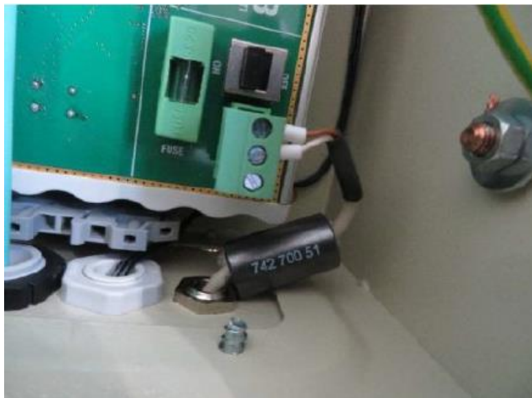
Ferrites 742 700 51 on the DC Power terminals of the COM HUB
