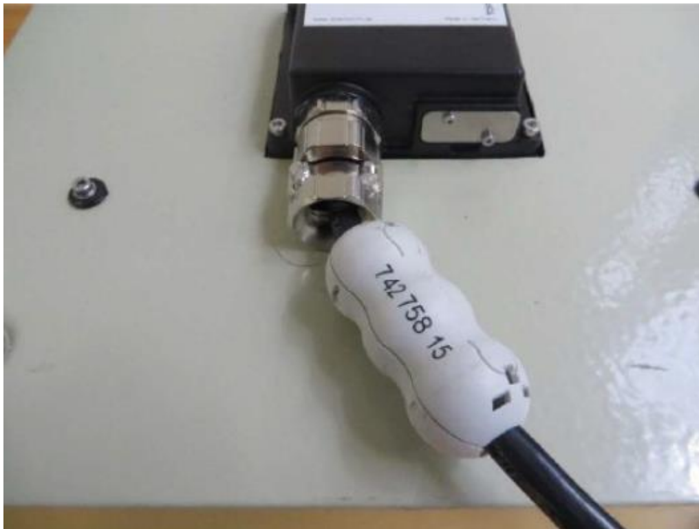
Snap-on ferrite 74275815 on the PLC J-Box side
