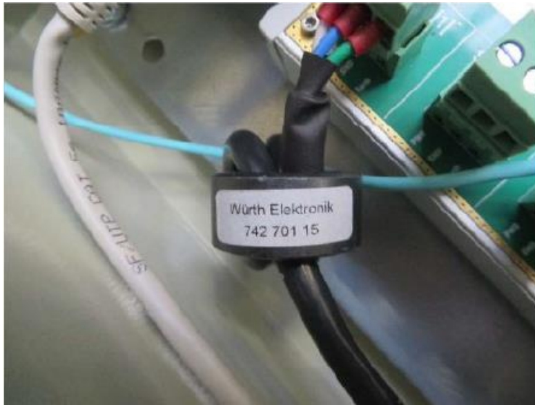
Ferrite 742 701 15 on the sensor terminals of the COM HUB
